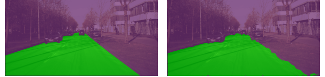
(a) Manually labeled data. (b) Prediction of binary DAD-Net.
